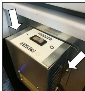
5 - Push in new switch. Make sure it is the right way round.
