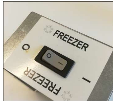
5 - Push in new switch. Make sure it is the right way round.
