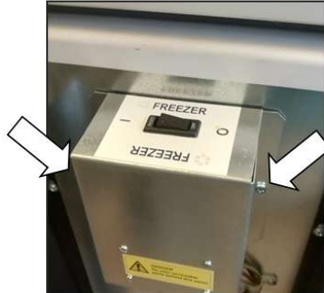
2 - Remove the 2 cover screws and keep safe.
