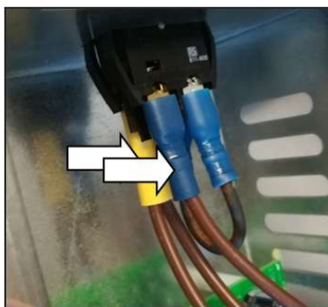
4 - Remove switch by squeezing at the sides.
