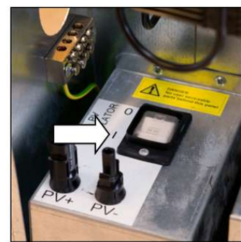
8 - Switch PV switch ON (1) and check that the freezer and freezer fan are working.
